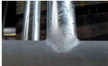
Example of permissible surface variations following hot-dip galvanising (Image source: Beuth-Verlag, Corrosion Protection: Hot-Dip Galvanising).
