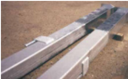
Example of permissible surface variations following hot-dip galvanising (Image source: Beuth-Verlag, Corrosion Protection: Hot-Dip Galvanising).
