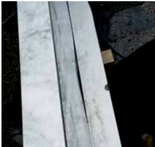
Typical local warping in flat, hot-dip galvanised elements. The warping is due to the manufacturing process and falls within the permissible limits set by the standard.
