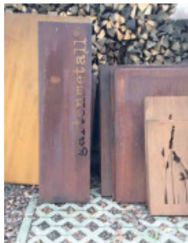
An example of rusted Corten steel in various shades.
