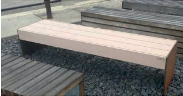
Example: Comparison of the greying of RESYSTA® and hardwood after approximately 24 months
